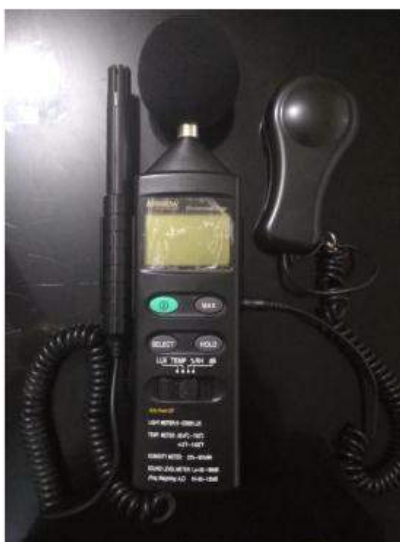
Gambar 7. Multifunction environment meter krisbow 4 in 1 KW06-291
